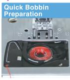
The bobbin preparation is easy. Just follow the guide and it is not necessary to pull up the bobbin thread.
