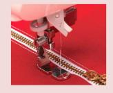
The position of the adjustable zipper presser foot can be changed over to the right and left of the needle to allow the sewing machine to sew the material while avoiding its thicker part such as a zipper.
